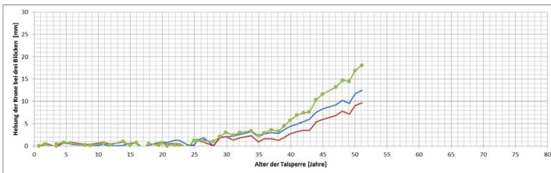
**Figure 42:** Long-term behavior of a rising dam at three different levels.
